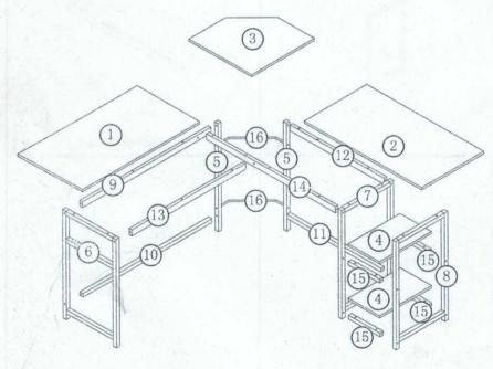
Notes:Don't tighten screws completely at first , just in case parts were assembled wrong and need disassembled. Tighten screws at last when all parts are put together.
